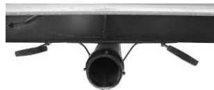
Black/Grey Tank Drain and Valves
